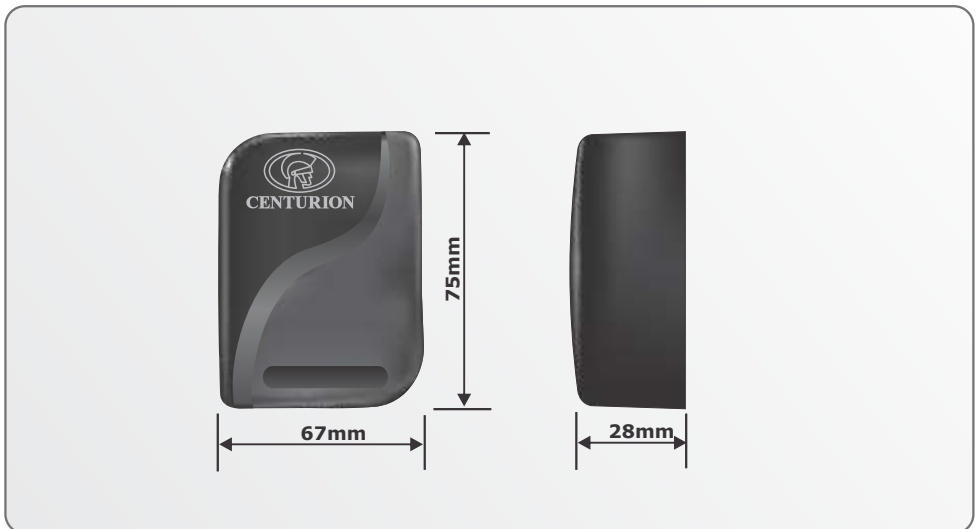
FIGURE 2. OVERALL DIMENSIONS FOR THE CP104 RECEIVER V3.1 (OR LATER)
